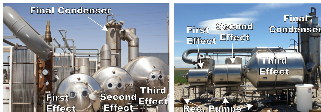
Fig. 4. Two views of the 3-effect plate-and-frame MED system used for the pilot demonstration before insulation was applied.
